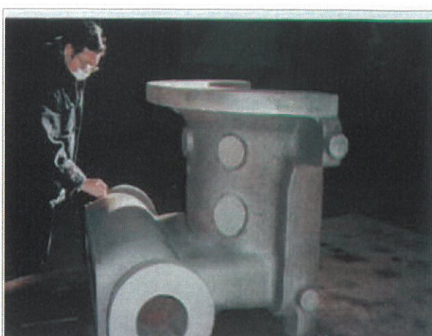
High Pressure Turbine Casing ,2500kg
