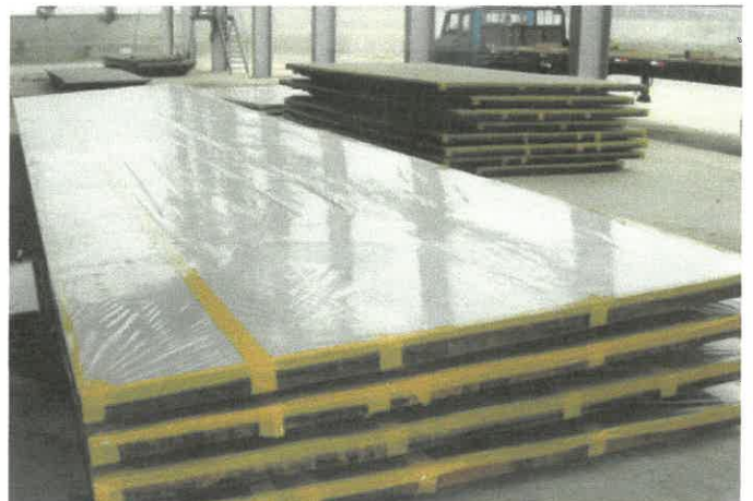
SUS/SS Clad (3+82)x2500 x12000mm
