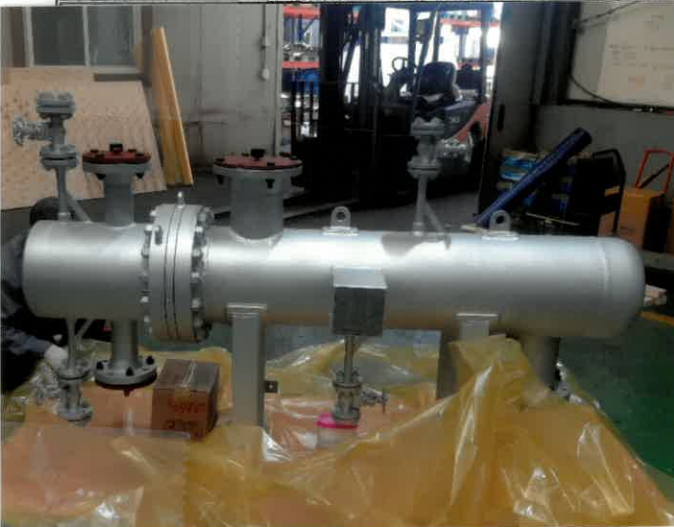
HEAT EXCHANGER ASME SA105 1940×600×1000H 単重 450kg
